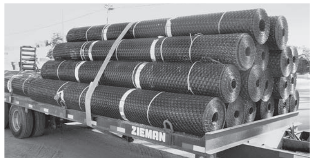
Storing the Tensar Geogrid rolls horizontally.
