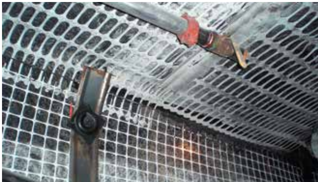
Tensor BX and UX Mining Geogrids provide effective roof and rib control for soft minerals as well as the most demanding hard rock and tunneling applications.
