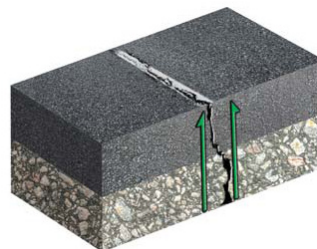
Figure 1 Cracks migrate toward surface in unreinforced overlay.
