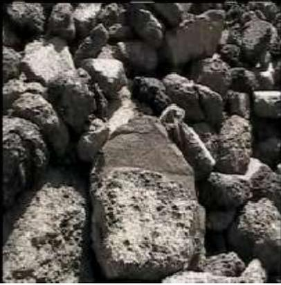
Larger pieces of asphalt are broken up when dumped into the recycled bin and larger pieces of fabric are discarded during this operation
