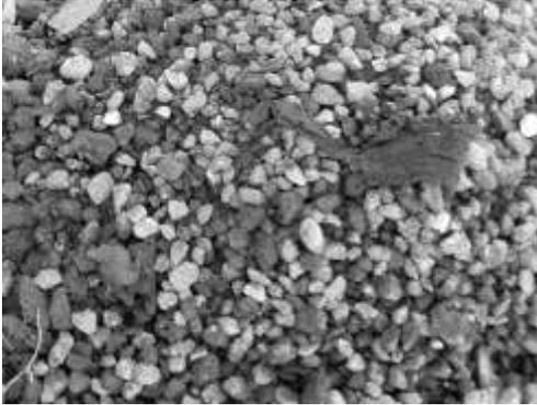
Rejected material on the right contains a small amount of paving fabric approximately 6 “ long and will not proceed to the drum dryer
