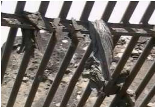
Stockpile material is dump into this large separator to eliminate chunks of asphalt and large fabric pieces from continuing on to primary crusher.
