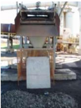
A secondary single deck-scalping screen vibrates debris and any visual pieces of fabric from the RAP entering the conveyor belt
