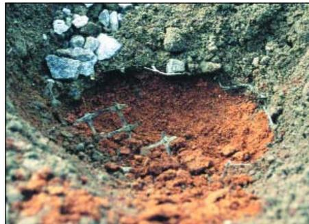
An excavation through the BX Geogrid interface shows that underlying red clay particles do not exist within the overlying well-graded aggregate base.
