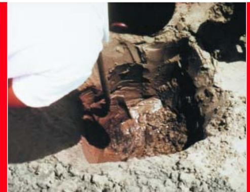
The excavation(s) at Westminster Levee revealed no contamination of black bayou mud within the light brown sand, all the way down to the Tensar BX Geogrid.
