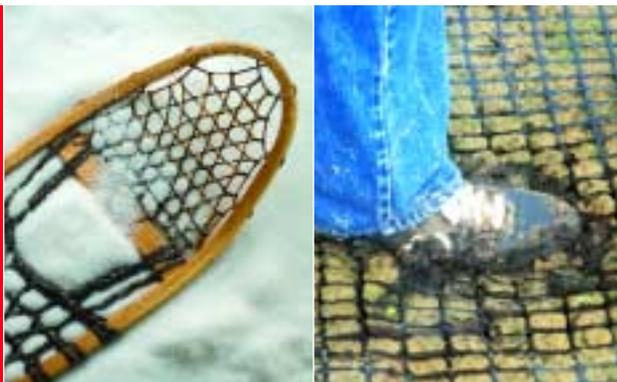
Snowshoe Effect — Tensar BX Geogrids distribute heavy loads over soft soils just like a snowshoe supports the weight of a man over soft snow.
