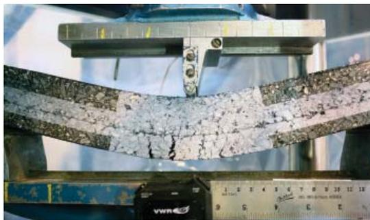
*GlasGrid TF provides a superior bond in the pavement cross-section to minimize cracking and maximize performance.*
