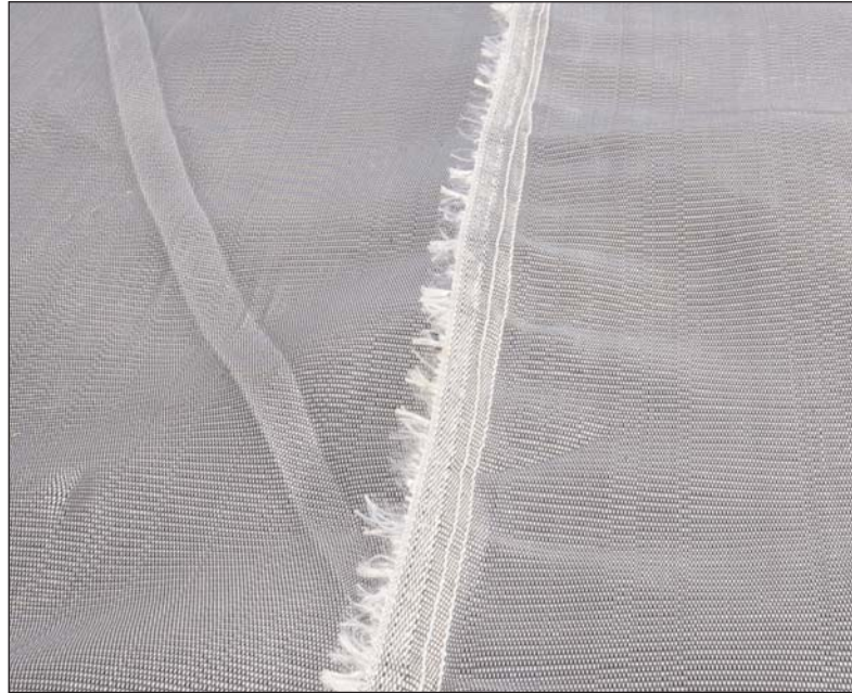
A prayer seam was used to stitch the panels of Geolon® HP770PET.
